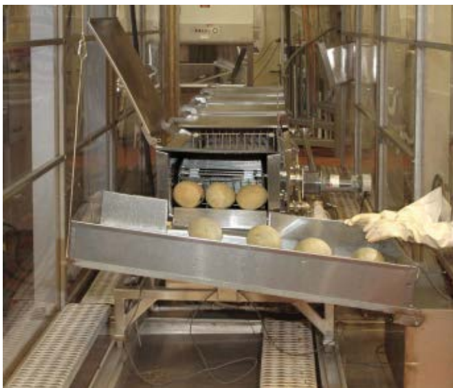
MELON MOVER — This commercial-scale pasteurization device can process up to 360 cantaloupes an hour. It submerges the melons in hot water to destroy pathogens on the rind.
