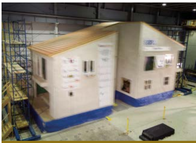
MOTION PICTURE — The blur in this image results from the shaking of the townhouse, not the camera. Researchers simulated a magnitude-6.7 quake to better understand how wood-frame structures behave in such temblors.
