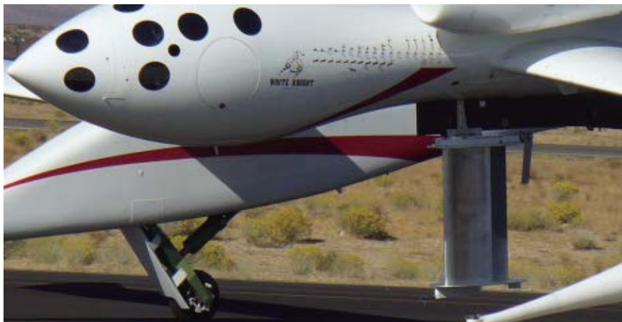
HANGING OUT A silver-colored wing prototype, mounted vertically beneath a jet, has a morphing trailing edge. Its developers completed flight tests of the novel wing last week.
