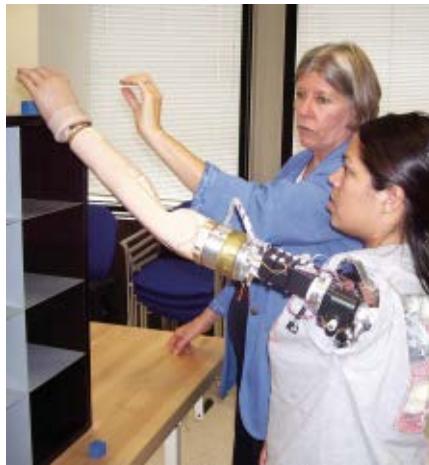
HELPING HAND Claudia Mitchell undergoes training to use her nerve-activated artificial limb. She is part of new research that may lead to prostheses that provide a sense of touch.
