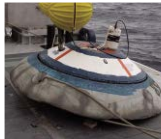
WATER METER A seafloor instrument like this one measured Gulf Coast currents as Hurricane Ivan passed overhead in September 2004.
