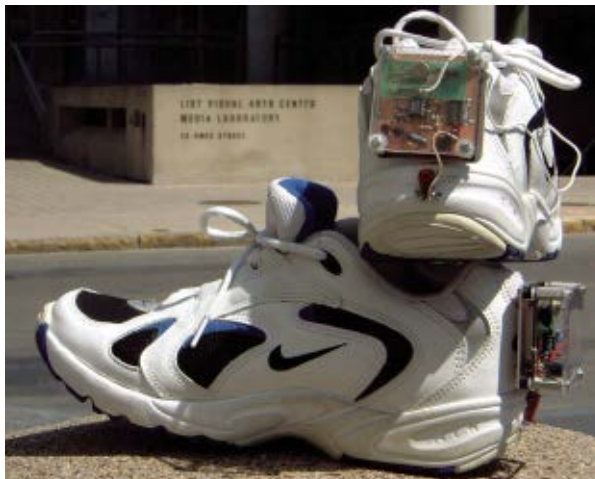
SHOE POWER — In an early experiment at the Massachusetts Institute of Technology, an energy scavenger built into the sole of a running shoe harvested about 60 milliwatts of the power a person expended while walking.
