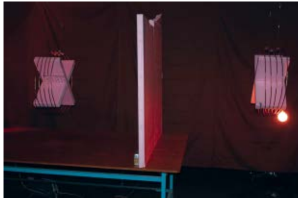
ABRACADABRA — The first demonstration of energy transfer based on magnetic resonance. The receiving circuit (right) picks up 40 percent of the power consumed by the emitting circuit (left) and lights the bulb.
