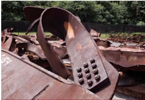
REMAINS OF THE DAY — Steel-beam remnants from the World Trade Center, contorted by fire on 9/11, lie in a yard at the NIST laboratories in Gaithersburg, Md. NIST scientists studied these beams in their investigation of the building’s collapse.
