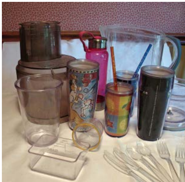
PLASTIC? OH NO — Plastic household products that are hard and clear are typically made of polycarbonate plastic, which tends to leach bisphenol A with age and after heating. When the plastic crackles, as often happens, the leaching accelerates.
