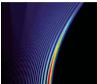
TURNING POINT A computer simulation shows that a laser beam tweaked by going through a liquid-crystal panel will take a curved trajectory. Experimental data confirmed the predictions.
