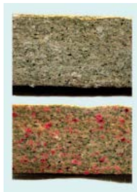
IN THE PINK Until treated, asbestos doesn't show up in cement (top). A new red-dye treatment can highlight even small traces (bottom).
