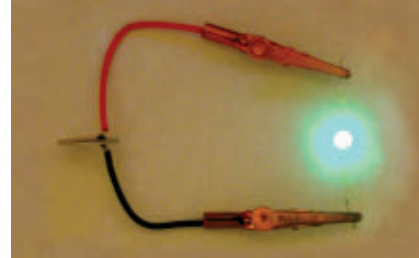
A battery with a cathode made from viruses turns on an LED.
