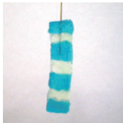
A new hydrogel (top, left) keeps its shape after soaking in a solvent (top, right), and blocks of the gel (blue and white, bottom) will bond to form a strong, larger structure.
