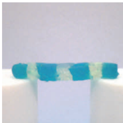
A new hydrogel (top, left) keeps its shape after soaking in a solvent (top, right), and blocks of the gel (blue and white, bottom) will bond to form a strong, larger structure.
