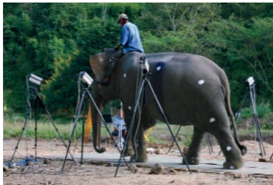
A 4-ton elephant named Tantawan crosses a force platform while cameras capture her movements.
