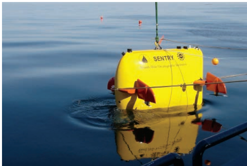
In June, researchers from the Woods Hole Oceanographic Institution probed an oil plume in the Gulf of Mexico using the SENTRY autonomous underwater vehicle.
