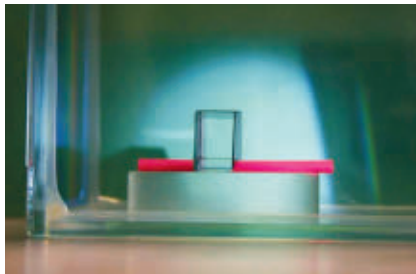
A piece of pink paper vanishes under a new invisibility cloak, made from calcite, that can hide macroscopic objects.
