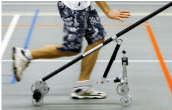
An experimental riderless bicycle has two extra wheels that spin backward. The bike demonstrates that the physics behind two-wheeled vehicles' stability is more complicated than researchers previously thought.
