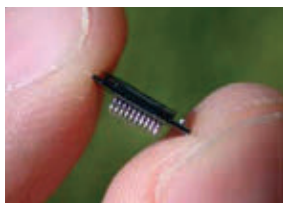
Wireless electrodes (prototype shown) may one day allow paralyzed patients to easily control a prosthetic device.
