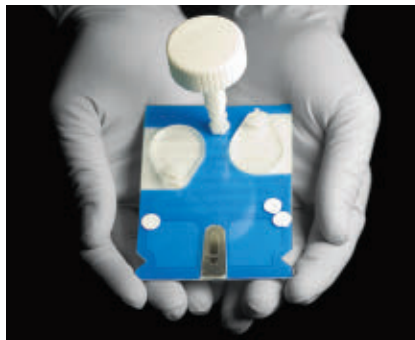
A dollop of saliva on a chip like this one can be analyzed for disease-related proteins by a portable detector.
