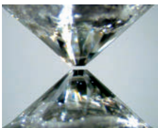
Here on Earth, scientists put on the pressure with a device called a diamond anvil cell.
