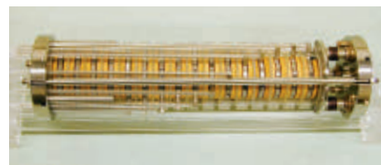
This trap captures protons emitted by neutron decay. Comparing the number of protons after a certain time to the initial number of neutrons helps scientists determine the neutron's lifetime.
