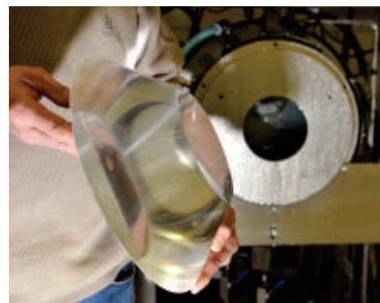
The Abyss Box, designed to house ocean dwellers at high pressures on land, weighs more than half a metric ton. The viewing window is about 10 centimeters thick.
