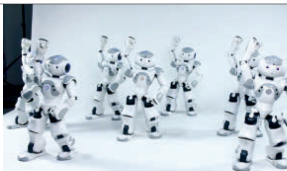
Sending information to and from an outside server keeps these robots in sync and even allows a robot that has fallen out of step to rejoin the group.
