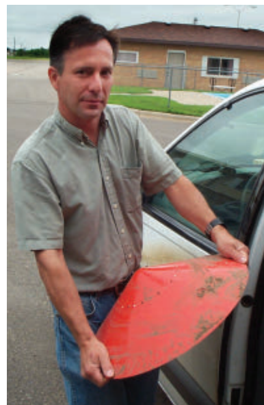
Tim Samaras holds one of the "turtle" probes that he designed to record pressure, wind speed and other conditions inside tornadoes.
