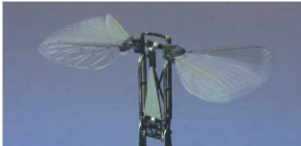
A robotic bee designed by Harvard researchers relies on a flat scaffold and more than 100 hinges. When the layers of the scaffold pop up, the bee takes shape and can be removed from its base.
