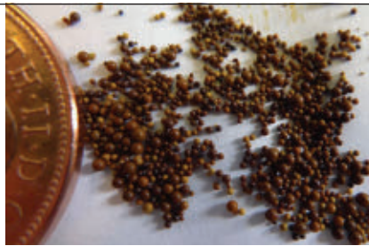
Inspired by arsenic-removal systems, one team has used tiny resin beads (shown) containing nanoparticles to strip phosphorus from wastewater.
