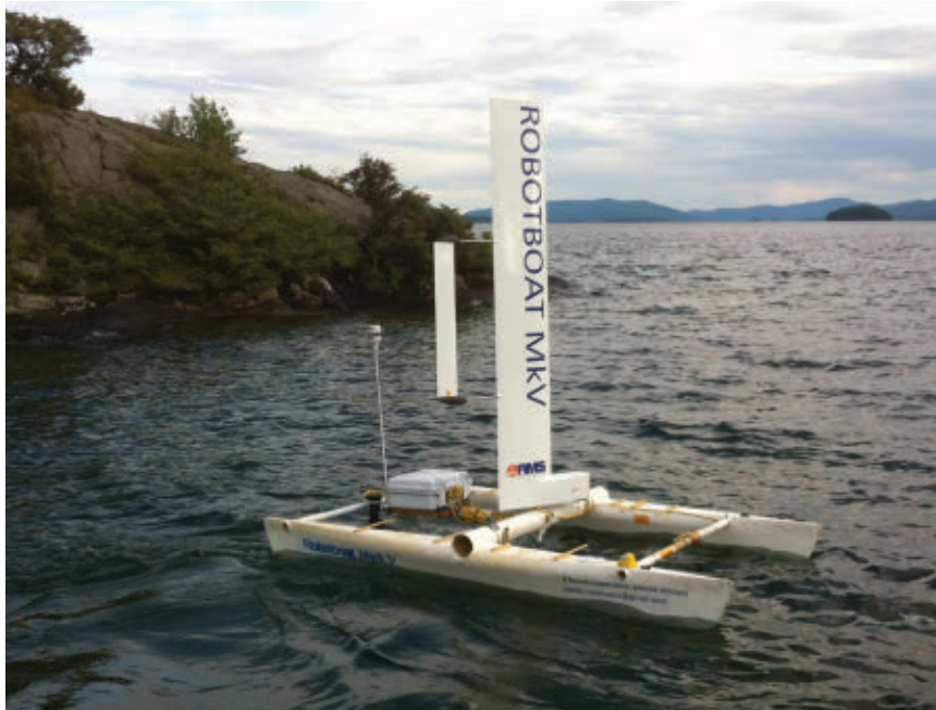
Engineer Walter Holemans envisions fleets of low-cost autonomous catamarans that could be used for collecting scientific data or patrolling remote waters for pirates or other dangers. He is testing prototypes made almost entirely of printed components.
