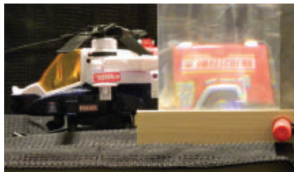
The rear of a toy helicopter is masked by a cloak made up of four glass lenses (front one shown). A toy truck placed behind the cloak appears instead.
