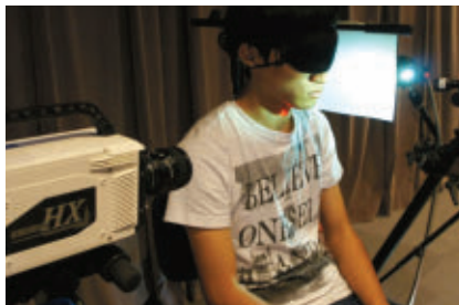
Using a high-speed camera to record neck vibrations, scientists can capture a person's voice without a microphone.
