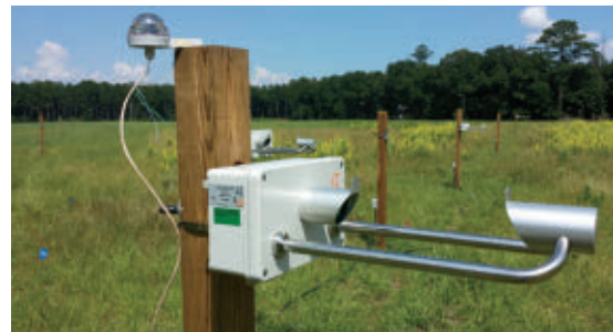
Researchers used an array of 22 sensors, including this one, to clock raindrop speeds.
