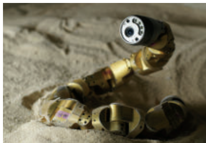
After researchers adjusted this robot's design based on studies of real snakes, the robot can now writhe up a sandy slope.
