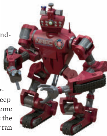
At 5 feet 2 inches tall and 400 pounds, this bot, called CHIMP, rolls on treads for extra stability. It can turn valves and operate power tools.
