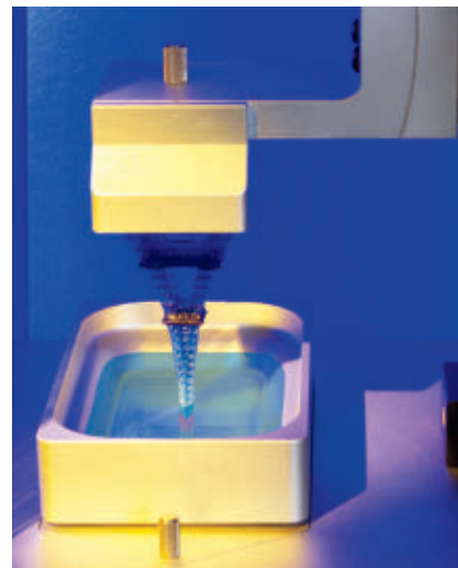
A mini-Eiffel Tower emerges from resin in just one hour, thanks to a new 3-D printing method that uses ultraviolet light and oxygen to create intricate objects.
