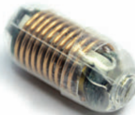
This 3.5-by-1.2-centimeter capsule can be swallowed to measure gut gases and send its findings to a smartphone. Researchers in Australia tested the device in pigs fed different amounts of fiber.
