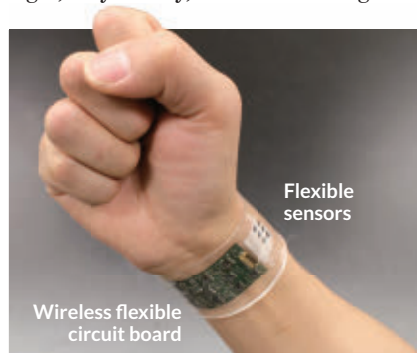
A new health device combines flexible sensors and an electronic circuit board to analyze sweat.
