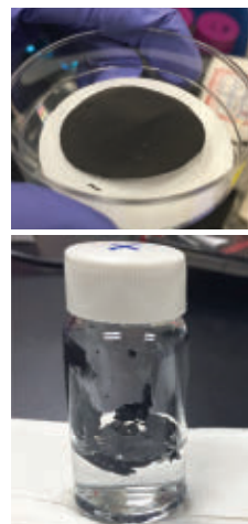
Researchers manufactured sheets of graphene oxide (top) that function as water desalination membranes. Each sheet contains many graphene oxide flakes (bottom) linked together.
