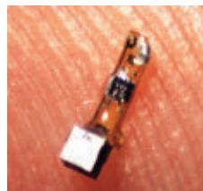
This tiny sensor that responds to ultrasound (shown on a fingertip) picked up signals from rat nerves and muscles.
