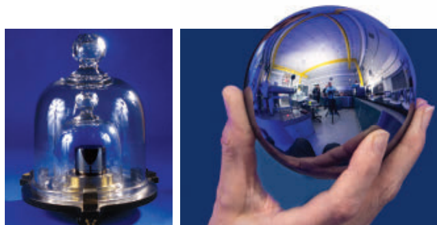
A kilogram cylinder replica (left) is safeguarded under bell jars. Ultra-smooth silicon spheres (right) will soon be used to redefine the kilogram using the Planck constant — making the kilogram prototype obsolete.
