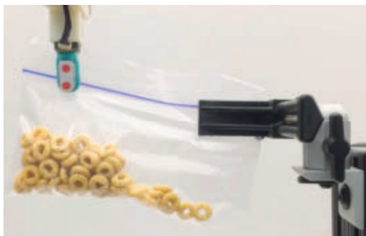
Deformable, sensing finger pads (green, above) help a robot figure out how to seal a plastic bag. Researchers at UCLA designed a learning algorithm that gives the robot points for keeping the seal in the center of the finger pad (green square, right).
