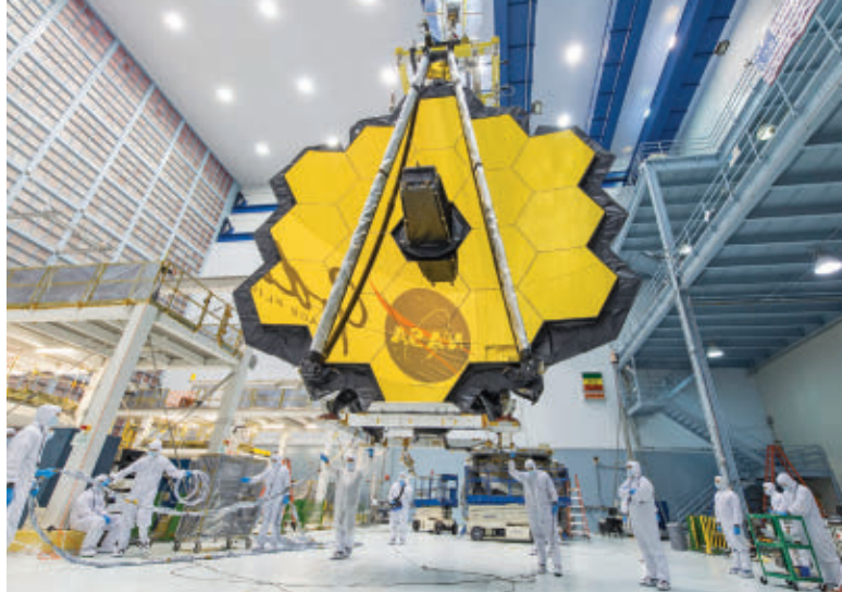
NASA's James Webb Space Telescope will study exoplanet atmospheres for signs of life. The 6.5-meter-wide primary mirror recently moved into a clean room at the Goddard Space Flight Center in Greenbelt, Md.
