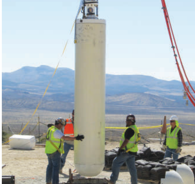
Technicians lower an enormous canister of explosives into the ground in southern Nevada for a chemical explosion — part of the Source Physics Experiment series — to mimic the physics of nuclear blasts.
