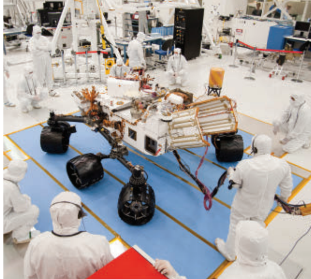
The Mars rover Curiosity was assembled and tested in a clean room before its 2011 launch, in part to limit the hitchhikers it carried from Earth.
