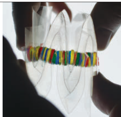
A polyester sheet with hydrogels (colored disks) printed in a precise configuration folds up so the hydrogels stack similarly to the cells in an electric eel’s electric organ.
