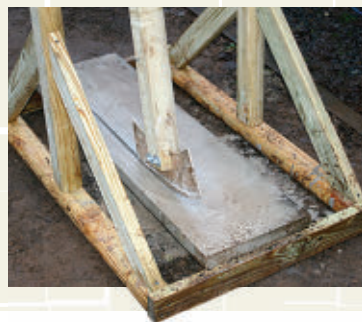
Archaeologist Nicholas Blackwell (top, left) and brother-in-law Brandon Synan operate Blackwell's reconstructed pendulum saw, using a rope to pull a blade-tipped wooden arm back and forth across a piece of limestone. An experimental bronze blade appears in action (left).
