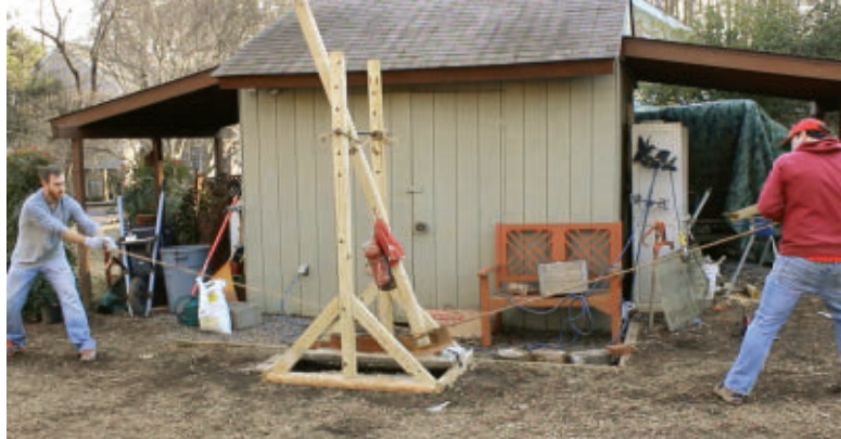
Archaeologist Nicholas Blackwell (top, left) and brother-in-law Brandon Synan operate Blackwell's reconstructed pendulum saw, using a rope to pull a blade-tipped wooden arm back and forth across a piece of limestone. An experimental bronze blade appears in action (left).
