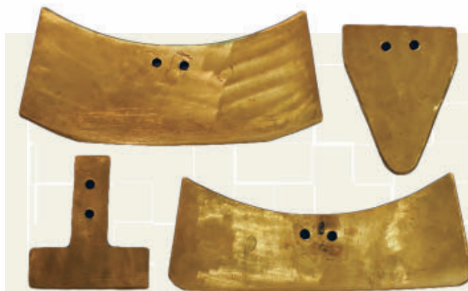
Stonecutting experiments with a model of a pendulum saw tested four bronze blades crafted in Crete for the studies. Blades on the top left and bottom right produced Mycenaean-style curved incisions in rock. A triangular blade, top right, created a wobbly groove. A short, straight blade, bottom left, repeatedly became stuck as it swung into a rock's surface.
