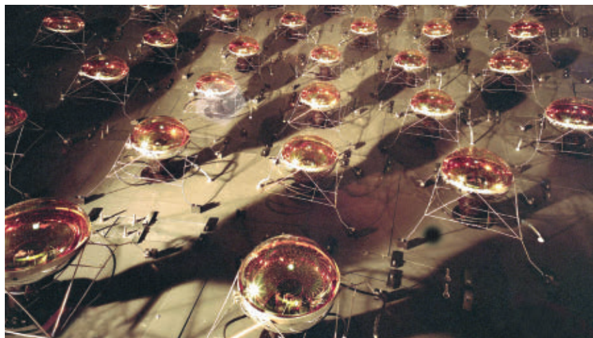
The MiniBooNE detector, a tank holding mineral oil and lined with light sensors (shown), looks for flashes produced as subatomic particles called neutrinos interact with atomic nuclei inside the oil.
