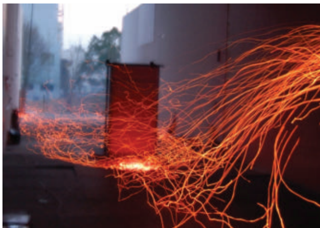
The "dragon," designed by researchers at the National Institute of Standards and Technology, shoots showers of embers to help scientists study fires in the laboratory. A time-lapse photo (bottom) shows the paths of embers moving through the air.
