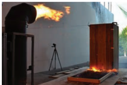
The "dragon," designed by researchers at the National Institute of Standards and Technology, shoots showers of embers to help scientists study fires in the laboratory. A time-lapse photo (bottom) shows the paths of embers moving through the air.
