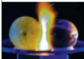
Plasma erupts when two grapes, or a grape and a hydrogel bead (shown), are heated in a microwave.
