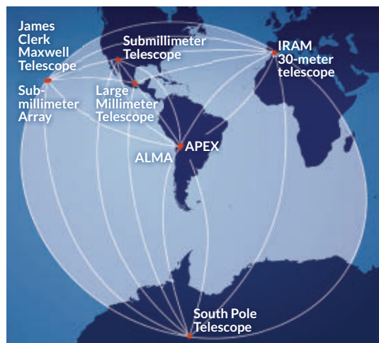
In 2017, eight observatories teamed up in the Event Horizon Telescope to peer at two supermassive black holes: one at the center of the Milky Way and one in galaxy M87. Combining data collected by pairs of telescopes allowed the network to act like one giant radio dish.
