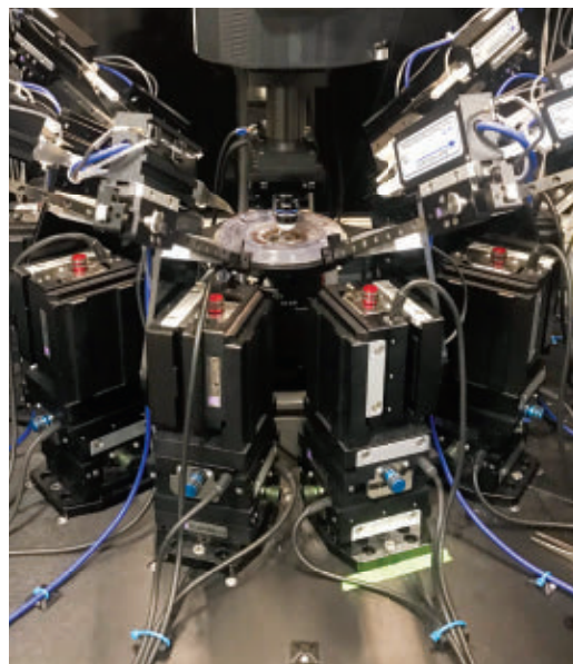
Using a multistation rig at the Allen Institute, researchers can observe a group chat among a handful of live neurons in response to an injected electric current.
