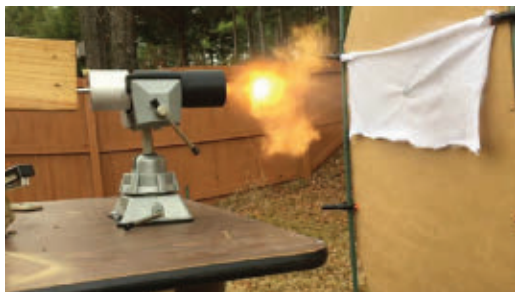
The University of Mississippi team sometimes used a machine to pull the trigger on 3-D printed guns, then looked for clues on bullets, cartridge cases and the target.
