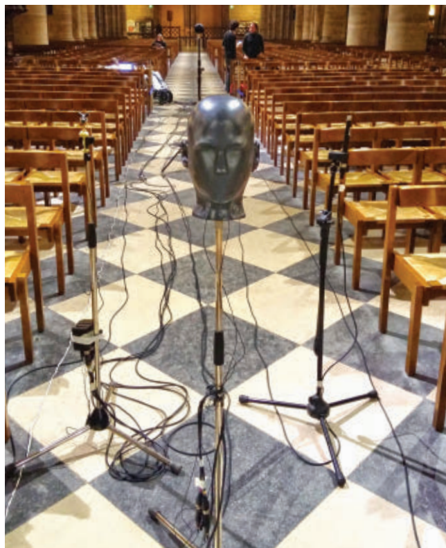
Brian Katz took detailed acoustic measurements in Notre Dame in 2013, using microphones on stands and a dummy head. These benchmark data will help reveal how rebuilding could alter the cathedral's sound.
