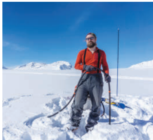
Glaciologist Andy Aschwanden drills an ablation stake, to monitor ice levels over time, into the Black Rapids Glacier in eastern Alaska in April 2016.
