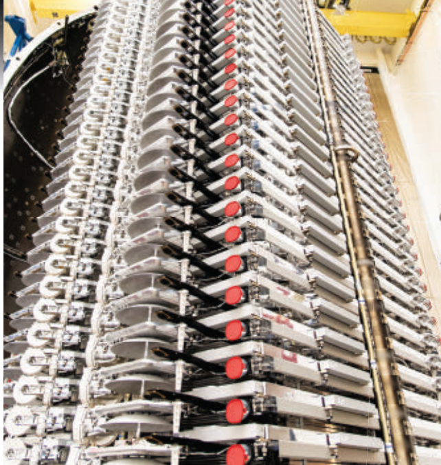
Starlink satellites are launched 60 at a time in stacks like the one shown here. The stack sits at the top of a rocket. Once in orbit, the satellites disperse around the planet.
