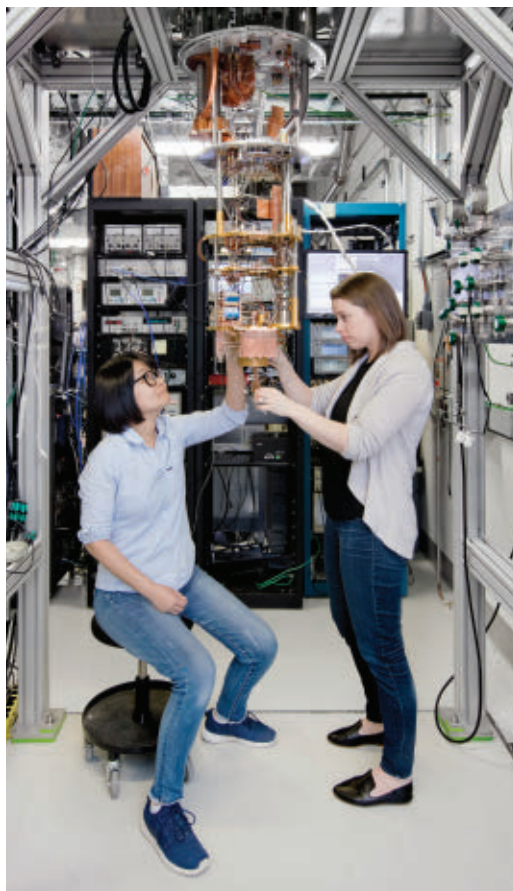
IBM researchers Hanhee Paik (left) and Sarah Sheldon (right) work on a quantum computer that is cooled by a hanging dilution refrigerator. IBM has made 18 quantum computers available for use online, and all grapple with errors.
