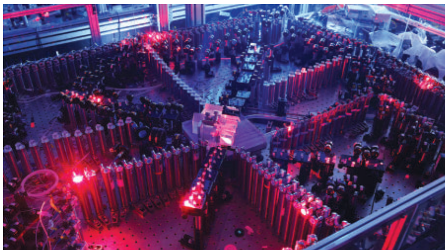
A new quantum computer manipulates light via an array of optical devices (shown on a table).
